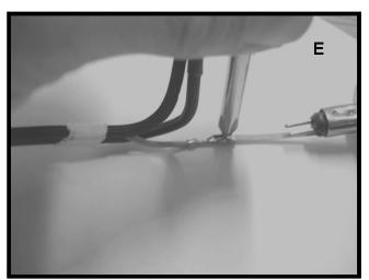
Place Phillips screwdriver in the center of the eyelet barrel and using Hammer spread the eyelet by hitting the top of the screwdriver to hold the brass eyelet in place. An extra eyelet is provided in case of loss.
