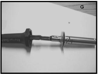
Slide handle over the base of the heating element and tighten in place using Allen Wrench.
