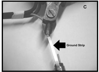
Snip head of eyelet using wire clippers. Make sure the barrel of the eyelet has been pushed through the hole in the ground strip & slide ground wire off ground strip. The old element can now be discarded.
