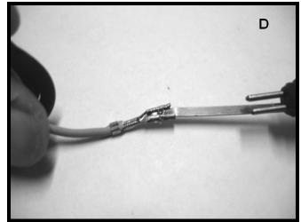
Slide brass connector on cord-set ground over the ground strip on the new element. Line-up the hole in the ground strip over the hole in the brass connector and slide over the new brass eyelets provided.
