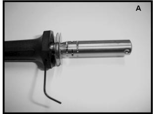
Using Allen Wrench, loosen set screw in handle enough to slide element apart from handle (Do not fully remove set-screw)
