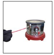
It is critical to maintain a level of operator consistency after the soldering process has been properly established. While it can be easy to become complacent, one must always remember that a solder pot maintains a bath of molten solder at temperatures as high as 900°F that can easily lead to serious injury.
