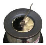
Use dross skimmer to remove residue that develops at surface of molten solder, prior to dipping any components or parts into the solder bath. Integrated skimmer moves dross onto the lip of the solder pot crucible where it dries up and can be easily removed.
