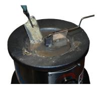
Solder should be replenished regularly by adding small amounts of solder that can quickly assimilate with the rest of the solder bath. This limits the temperature variation caused by adding large amounts of solder at one time.
